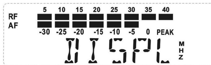
On the receiver you can choose whether the frequency or the channel number will be displayed in display. Select the “DISPL” menu by pressing the “SET” button. With the “▲” or “▼” buttons you can choose between: channel number: “CHANNEL” or frequency: “FREQU” After selection display starts flashing, at this moment press SET button to record your settings. Press SET button one more time to return the main display.
