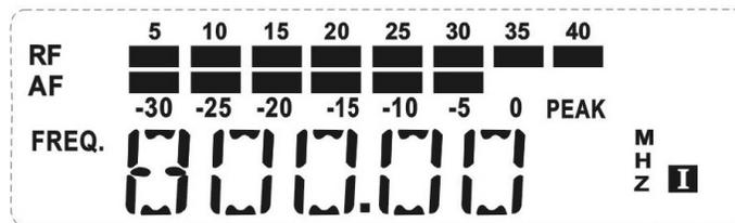
With the “▲” or “▼” buttons you can directly switch between the factory-preset frequencies (Channels presets). The display starts flashing by indicating that your selection is active. Press SET button to record your setting.
