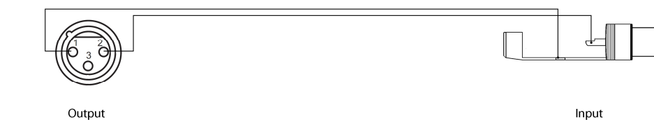
Cable to RCA input from balanced output. RCA and XLR connectors.
