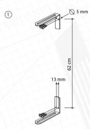
Fix mounting bracket on solid surface (recommended distance between brackets center holes 62cm)
