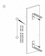
Fix mounting bracket on solid surface (recommended distance between brackets center holes 340 mm for COM SLIM 30 and 740 mm for COM SLIM 50)
