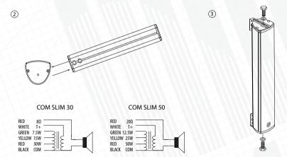
Remove the bottom cover and install the cable glands. Insert the cable into the cable gland and connect the cable to terminal block. Select desired power from table (transformer power tap meanings and wire colors are marked on the label). Close bottom cover.
