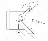
Remove mounting bracket from loudspeaker.
