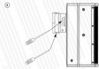
Plug audio cables and make final loudspeaker angle adjustments. Place the screws for fixing vertical and horizontal angles and tighten.
