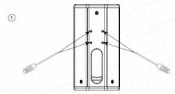
Unscrew four sockets on the back of loudspeaker. Do not use these removed screws for mounting - proper size screws for attaching bracket are included with RF UB.
