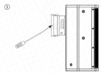
Place loudspeaker with attached bracket onto mounting plate. Fix the two security screws on both sides of the bracket to prevent loudspeaker removal from the plate.
