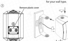
Remove plastic cover . Place loudspeaker to the bracket and tighten by bracket knobs. Connect Euro block connector to socket. Set the desired loudspeaker power tap.
