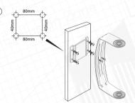
Drill holes according the drawing.
