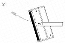
Place loudspeaker into the bracket and tighten the screws on both sides. Plug audio cables and make final angle loudspeaker adjustments.
