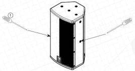
When mounting RF 6 vertically, unscrew sockets on the sides. Do not use these removed screws for mounting - proper size screws for attaching bracket are included with V6B.
