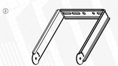
Attach mounting bracket to the surface. Please leave required space from all sides for cables and loudspeaker angle adjustment.
