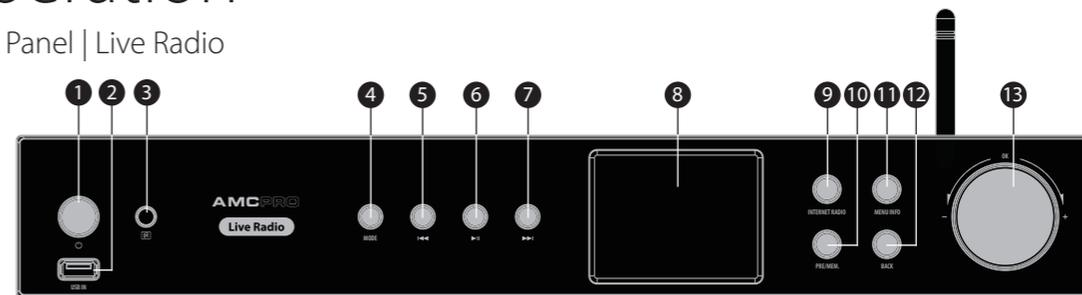
1. Power switch | 2. USB port | 3. Remote control sensor | 4. Mode | 5. Backward | 6. Play/Pause | 7. Forward | 8. Display | 9. Internet radio | 10. Preset | 11. Menu/Info | 12. Back | 13. Menu navigation and volume control
