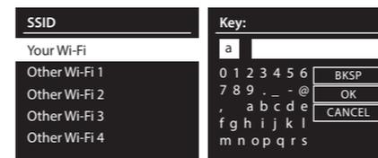
Backspace, OK, and Cancel are located to the right of the password screen. These menu options can be achieved using the rotary encoder or pressing the MENU/INFO button. The MENU/INFO button allows an instant jump to the Backspace option and back again.
