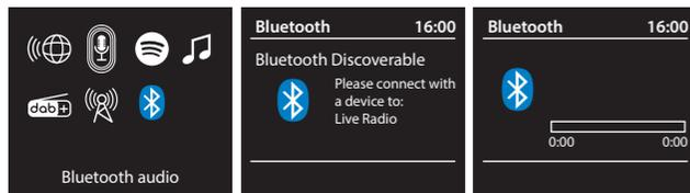
**Pairing Bluetooth:** The flashing Bluetooth icon indicates that receiver not paired to the Bluetooth device. To pair, select the option to add a new Bluetooth device on your smartphone according to your smart device instructions. Live radio will be displayed on the list of available devices that appear on the mobile device screen. Your mobile device will connect automatically once pair. After pairing Bluetooth icon stops blinking.
