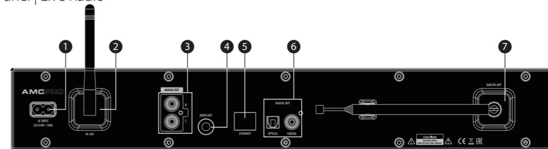
1. Main power plug | 2. WiFi antenna | 3. RCA audio output | 4. 3.5mm audio output | 5. LAN cable socket (RJ45) | 6. Optical & Coaxial output | 7. DAB/FM antenna
