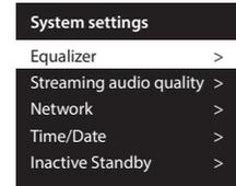
**SYSTEM SETTINGS.** Menu allows setting all main live radio parameters. These settings are available from any other Live radio menu, usually located at the end of other menu choices. Press and hold the menu/info button and use the rotary encoder to scroll and find the system settings menu.
