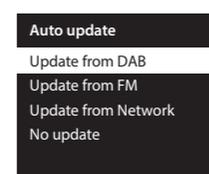
**Auto update:** Live radio can synchronize the time and date by using a control signal from the FM, digital radio, or network signal. To specify the clock synchronization options enter to Auto update menu and press the rotary encoder to choose between the ‘Update from DAB’, ‘Update from FM’, ‘Update from Network’, and ‘No Update’ clock synchronization options.
