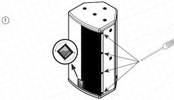
When mounting RF 6 horizontally, AMC logo and horn (tweeter) can be rotated sideways. Unscrew loudspeaker grill and loosen the screw holding the logo plate. Unscrew the horn to rotate it.
