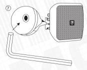
Use the hexagon key to tighten bracket angle adjusting screw.
