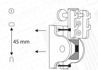
Drill the holes according to the drawing.
