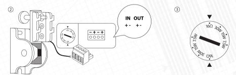
Connect the audio cable to the Euro block connector and the socket.
